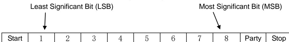
Transmit Character = Start Bit + Data Byte + 2 Stop Bits (11 bits total):
