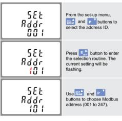
On completion of the entry procedure, press 🛃 button to confirm the setting and press [V/A] button to return the main set-up menu.
