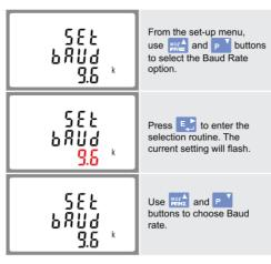
On completion of the entry procedure, press [ to confirm the setting and press [1/4] to return to the main set up menu.
