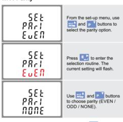
On completion of the entry procedure, press 🔁 to confirm the setting and press V/A to return to the main set up menu.
