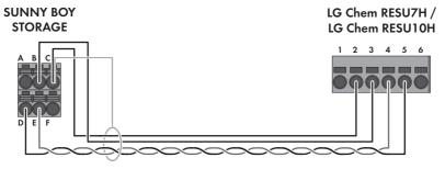
Figure 1: Cabling plan SBS2.5-1VL-10 with RESU7H / RESU10H
