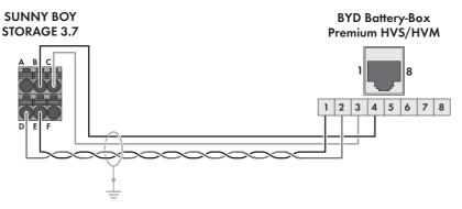
Figure 6: Cabling plan SBS3.7-10 / SBS5.0-10 / SBS6.0-10 / SBS3.8-US-10 / SBS5.0-US-10 / SBS6.0-US-10 with Battery-Box Premium HVS or HVM
