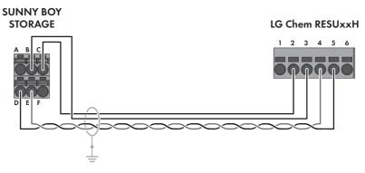
Figure 3: Cabling plan SBS3.7-10 / SBS5.0-10 / SBS6.0-10 / SBS3.8-US-10 / SBS5.0-US-10 / SBS6.0-US-10 with RESU7H / RESU10H
