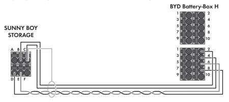
Figure 2: Cabling plan SBS2.5-1VL-10 with Battery-Box H
