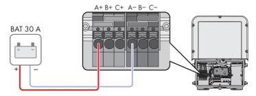
Figure 9: Overview for connection of one battery with a charging/discharging current higher than 20 A.
