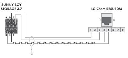
Figure 4: Cabling plan SBS3.7-10 with RESU10M
