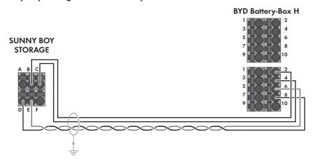
Figure 5: Cabling plan SBS3.7-10 / SBS5.0-10 / SBS6.0-10 / SBS3.8-US-10 / SBS5.0-US-10 / SBS6.0-US-10 with Battery-Box H  $\,$
