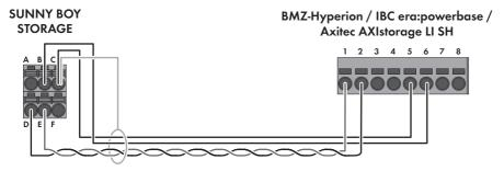
Figure 7: Cabling plan SBSxx-10 with BMZ Hyperion, IBC era:powerbase and Axitec AXIstorage Li SH
